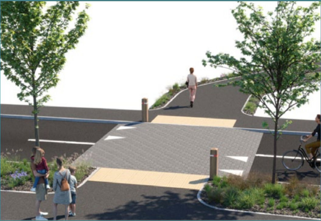
RAISED TABLE TO PRIORITISE PEDESTRIAN & CYCLIST CROSSING - EXAMPLE FROM SUFFOLK STREET DESIGN GUIDE
